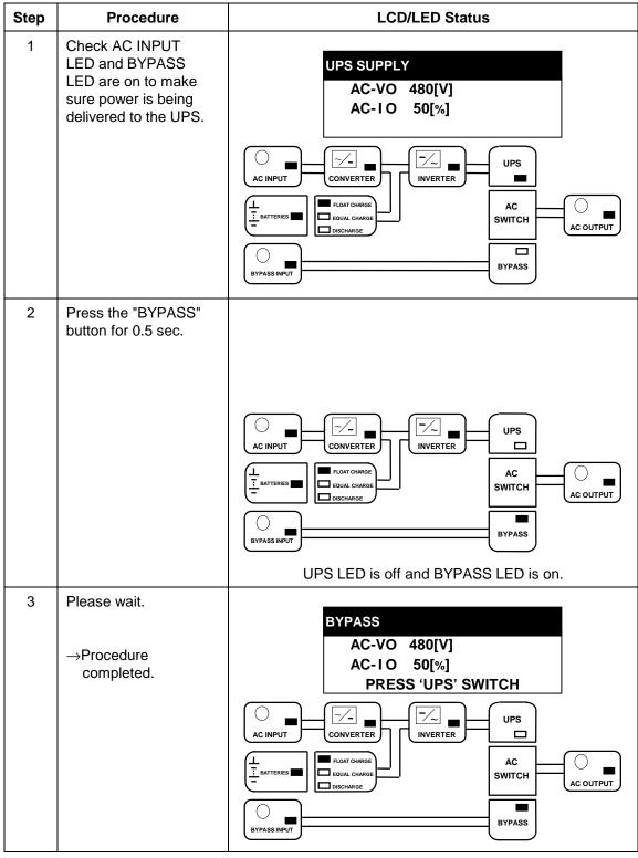
\* To change from Bypass to UPS supply, follow the procedure step #5 in Table 13. If the AC switch does not function, contact Toshiba or authorized representatives.
